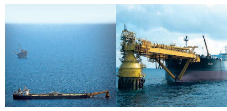
The Vega oil field is located in the Strait of Sicily, 20 kilometers off the Pozzallo (RG) coast. The facilities include a platform (Vega A), built on eight legs in about 120 meters of water, and the Leonis Floating Storage Offloading (FSO) vessel.
